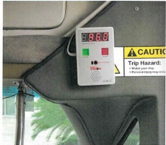
Using a high-precision temperature measurement sensor imported from Belgium, Safety Vision's IR thermometer measures the human body surface temperature without any contact. When an abnormal body temperature is detected, an audible voice warning will occur. This can be used as a stand-alone product or integrate with walk-through metal detectors, doors, intelligent access control systems, and more.
