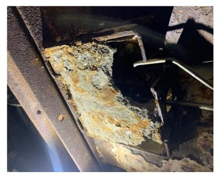
When this goes unattended for a period of time, the accumulated dust and dirt can form a substance very similar to concrete as shown in the photo above. This basically ruins the fuel tank supply valve which will require replacement.
