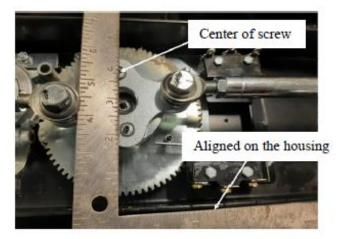
6. If the pivot is oriented correctly, the bottom screw is slightly skewed to the right as shown below.
