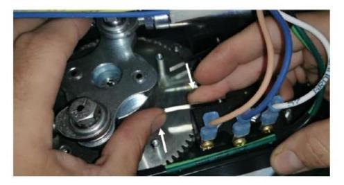
4. Open and close the door using the console switch. Verify the orientation of the pivot. If the orientation is correct, proceed to the door adjustment. Otherwise, repeat Point 3 until the pivot is oriented correctly.
