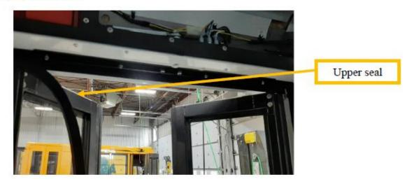
2. Use the console switch to close the door. Make sure that the door panels do not touch the doorstep nor top frame. If the door is still pressing the frame, give some more clockwise turns (toward you) on both rods, making sure that they have received the same number of turns. Verify and repeat in case there is still contact.
