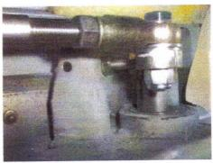
5. We suggest you use fish scales to test the handle. Weight to release the emergency door handle should not be more than 10 pounds. The leaves must close with electric power. If they are not doing so, you will have to adjust properly (check first step on page 1).
