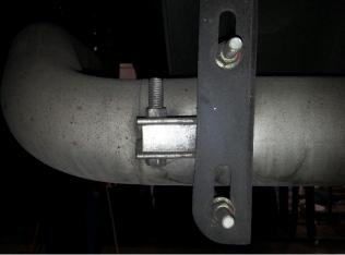
New York Bus Sales has also taken the step of adding Stainless Steel u-bolt saddle clamps to their inventory as an alternative to purchasing the standard steel to help deter the process on your units!
