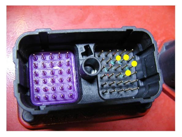
PLEASE NOTE – We would have recommended that when performing Service Bulletin S10SA for Low Coolant Sensor Leaks that you remove the "mats" to inspect the base of ALL pins on the ECM, but seeing as this has expired we recommend that if issues occur with the units that fell under this Bulletin that the inspection is performed just to assure there are no issues-
