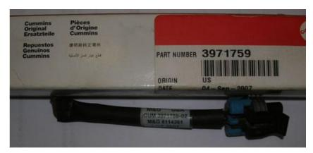
1/14/2012 - The original WIF sensor has been replaced. The replacement uses a better potting compound to prevent water from "wicking "along the wires and giving a false indication of water in the fuel.
