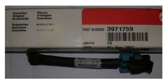
Pictured above is the tool Cummins offers to check the <u>Water-in-Fuel</u> sensor and circuit. We all know how sensitive today's electronics are to fuel and oil contamination. All you do with this handy tool is unplug the sensor and the plug this into the harness. You cycle the key off and wait one minute then turn the key back on and wait another minute and if the light goes
