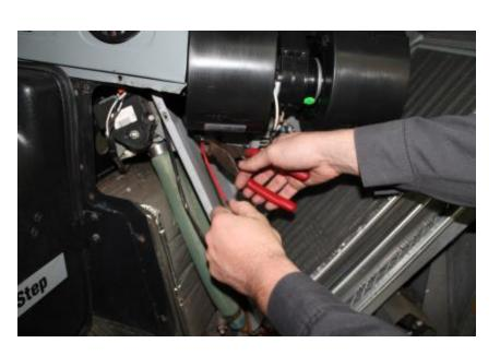
Tape wire back into the harness with electrical tape
