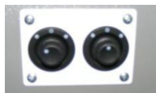
Heated mirror defrost switch: Allows the driver to activate heat in mirrors.
