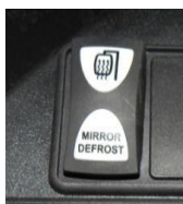
Heated mirror defrost switch: Allows the driver to activate heat in mirrors.
