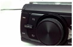
2 Remove the stereo faceplate. Using the tip of a ball point pen, press and hold down the [RESET] button for 5 seconds.
