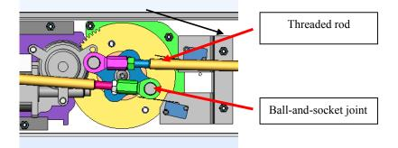
Adjust the stop bolt of mechanism with a  $\frac{1}{2}$  " wrench to keep the leaves open.
