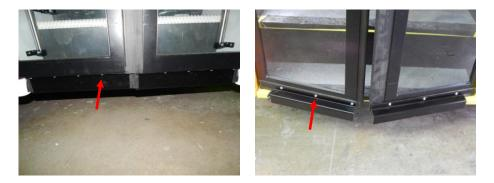
b) Using a Phillips screwdriver, remove both screws (up and down) on the door frame, which are holding the seals in place.
