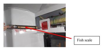
6. After you have adjusted & tested the door leaves operation, tighten the threaded rod nuts using a 9/16" wrench.
