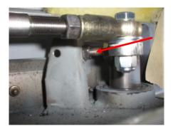
5. We suggest you use a fish scale to test the handle. Weight to release the emergency door handle should not be more than 10 pounds. The leaves must close with electric power. If they are not doing so, you will have to adjust properly (Refer to the beginning of step 2).
