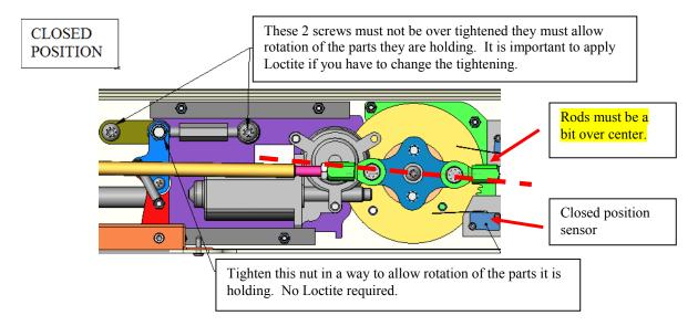
2. Align the gear with the mechanism in closed position. Adjust the closed position sensor to stop the gear at the indicated position. Bend the sensor strip to adjust the sensor.
