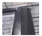
Step 2 : Remove protective tape and glue the bubble seal on the flat part of the flap which will be sitting on the rear door rubber.
