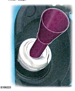
2. Insert the plastic funnel into the fuel tank filler pipe opening.
