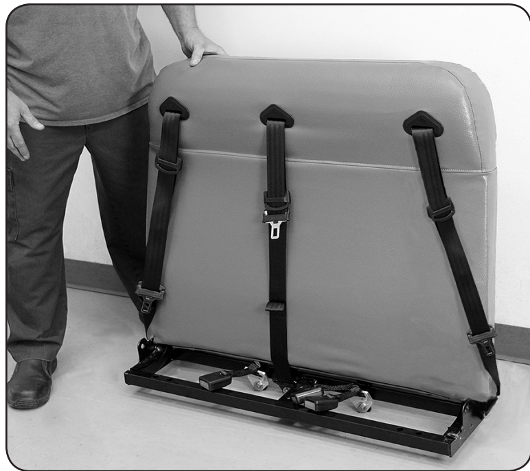
The Back Assembly with Cushion Assembly removed
