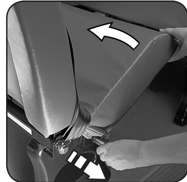
. . . pulling outward, lift the front of the cushion slightly.
