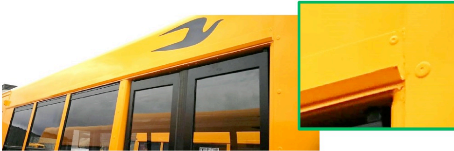
Figure 2: The esthetical aspect of the raised drip rail, now unsealed at the bottom
