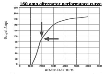
The typical School Bus today would require a 185 amp alternator to ensure that basic amperage requirements are exceeded and healthy batteries are maintained and would not be adequate if air conditioning were installed in all cases.
